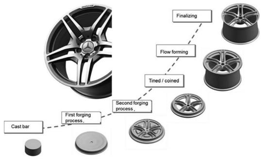
Fig. 2. Forging process [11]
