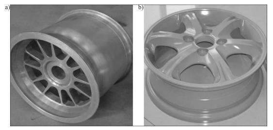
Fig. 4. AZ80 magnesium wheel (a) Magnesium alloy forgings [43], (b) Mg alloy wheels extruded (14×6) J [8]
