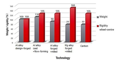
Fig. 1. Weight/rigidity comparison of certain wheel materials and technologies [2]
