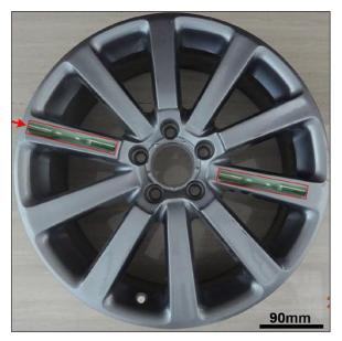
Fig. 3. Magnesium wheels of the Mg-2.96Nd-0.21Zn-0.39Zr [42]
